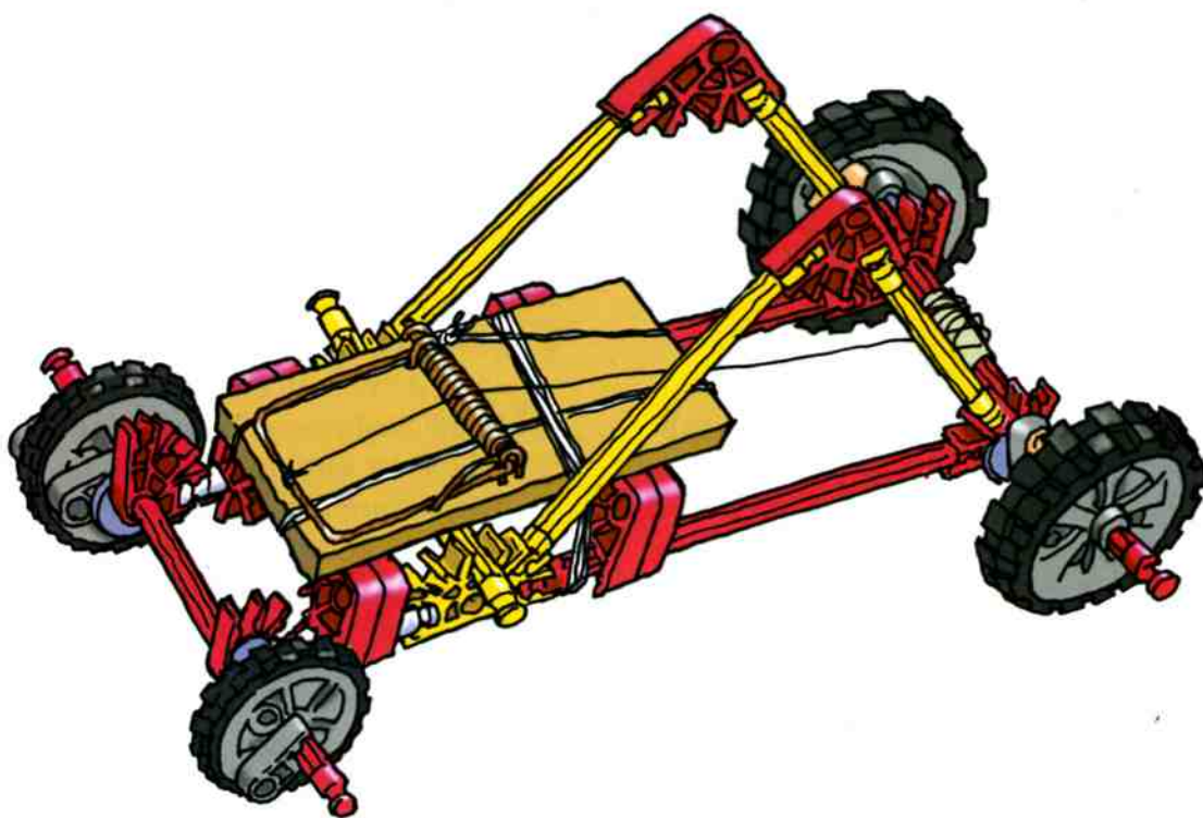
Figure 19.2 Assembled mousetrap car. The mousetrap in this illustration has been sprung. The string is attached to the jaws of the trap and to the rear axle. By turning the wheels, you can wind the thread around the axle and pull the jaws of the trap open.
